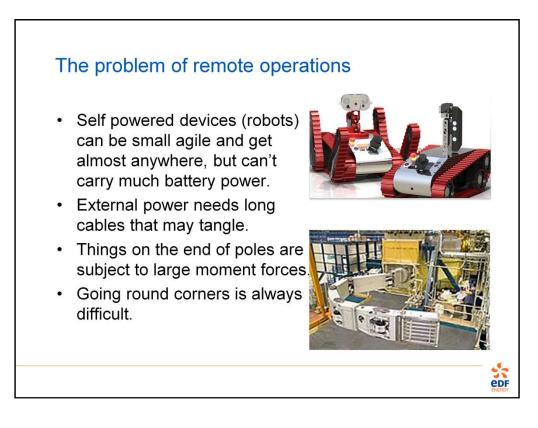
The bottom picture is the remote operations arm used in the Joint European Torus nuclear fusion project at Culham.
