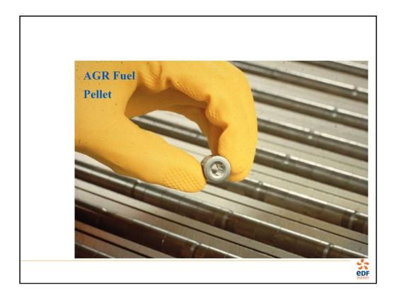
This is the inside of a pin - a fuel pellet. It is a ceramic – Uranium dioxide – which means that it can withstand very high temperatures before melting.
